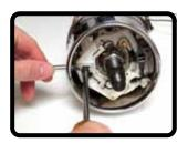
The turn signal lever installs into the left-side hole of the column and attaches to the white self-cancelling mechanism with the provided screw. Do not over tighten.
